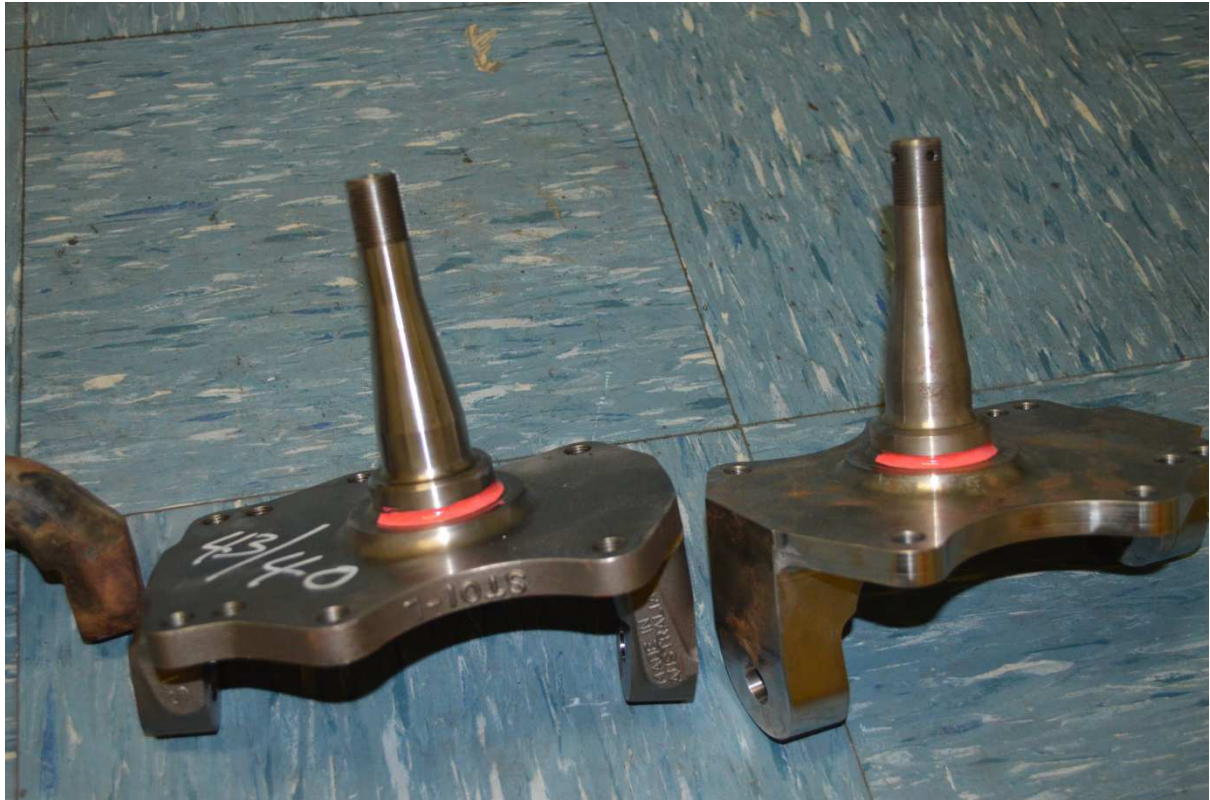
Figure 2. Position of cut on spindle.
